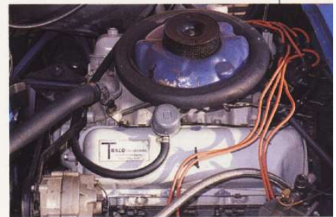
Top: The instrument panel of the Grand Sport is stock Corvette, with the exception of the 200-mph speedometer and the absence of heater controls and a radio. Carpeting, however, has been retained. Above: The 002 Grand Sport is currently equipped with a cast-iron 454-cu.-in. engine built by Traco. It, too, has a Holley carburetor.
