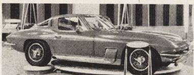
GRAND SPORT was late '63 racing effort which put lightweight body onto tubular frame. Result was a hairy, husky bear of a car. Later modification removed top.
