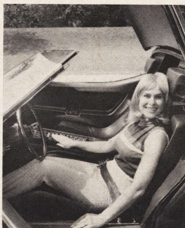
FLIP-TOP lid operates electrically but can be removed to make Mako an open car.
