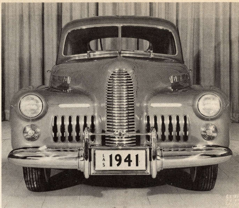
"Catwalk cooling", the routing of incoming air through side slots instead of grilles, is suggested by the stillborn 1941 LaSalle, above. Much later, GM Styling revived the general feeling of that design with the 1955 LaSalle II.
