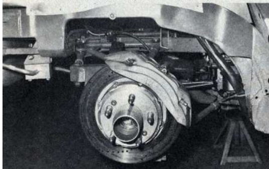
Race car's rear suspension has unequal-length A-arms.
