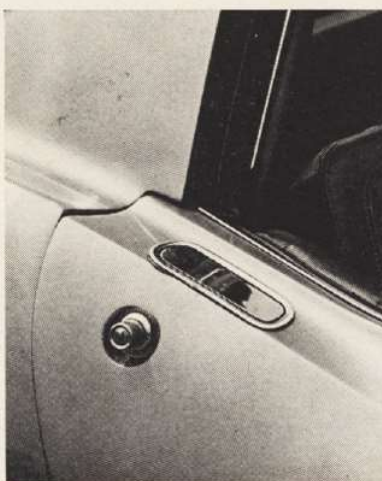
TO open, fingers push aside spring-loaded flap, thumb pushes button.
